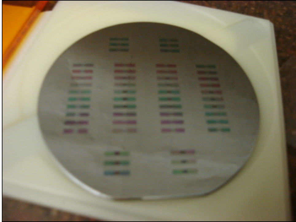
Figure 4-3. SU-8 patterned silicon wafer
